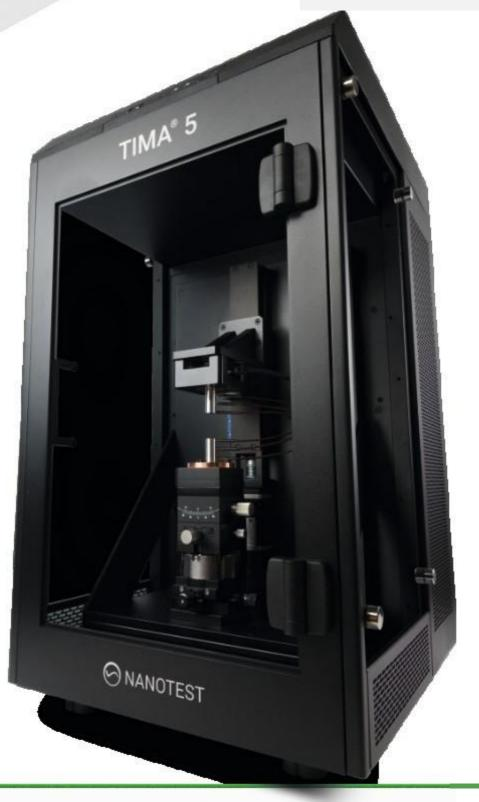
Thermal Interface Material Analyzer Model 5 The first convenient automated all-in-one ASTM D5470 test system.
